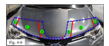
(f) Remove the solution from this section using upward and downward strokes (Fig. 4-6). Be sure that alignment of the lower edge is kept within proper tolerance dring the process. A small amount of alcohol solution may be used under the lower edge to esure placement is kept during the process.
