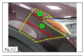
(b) Starting at area A, push the solution down around the headlight and out through the lower front edge to secure the film. Apply alcohol solution underneath the lower corner if needed to ensure placement is kept during process (Fig. 6-2).
